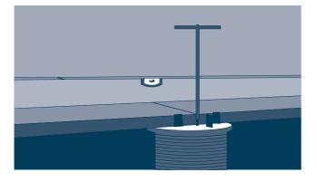
With the use of the special adjustment key it is possible to obtain a perfectly stable surface and with the required slope for better water drainage.
