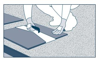
Position the tile and then compact the edges in order to level the tile with the substrate. It is suggested to use a joint of at least 4 mm to allow good water drainage.
