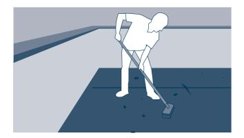
The installation on the plastic supports must only been done on perfectly waterproof substrates. Before proceeding with the installation clean the substrate thoroughly.
