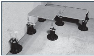
The stainless steel tile edge clip prevents contact between the tiles and the external perimeter wall and gives stability to the flooring. It is equipped with a dampener for longitudinal and transversal expansion and a safe hooking system to allow a linear and elegant perimeter joint.
