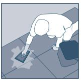
Once the installation is finished grout the flooring. Remember to observe the times indicated by the manufacturer for light foot traffic before walking on the tiles. "Post-installation" cleaning is mandatory at the end of the work and is required to remove residues of cement, lime or grout used for laying and filling the joints.
