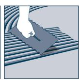
Before proceeding with the installation clean the substrate thoroughly. In order to obtain a flat floor, it is important to apply an even layer of adhesive.
