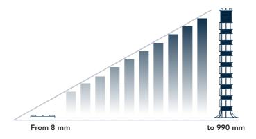
The structure of the supports consists of a base (which rests on the slab), a central screw adjustable in height and a head (on which the tile rests) which can be fixed or self-levelling with a self-adjustment system to alter inclination by up to 5°.
