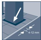
Around fixed elements of the supporting structure, such as walls, steps, columns, etc., it is mandatory to provide peripheral joints with a width of between 4 and 12 mm.
