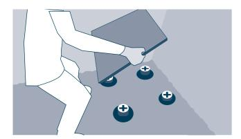
With regard to the number and position of the supports, as well as the type of reinforcement on the back of the slab, it is recommended to follow the instructions given in the following table, which are essential to evenly distribute the load.
