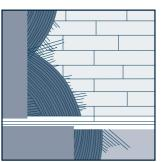
In correspondence with a structural or dividing joint in the screed, it is mandatory to provide an expansion joint with a width that is at least the size of the existing one. If there are joints between different surface types, it is mandatory to provide an expansion joint.
