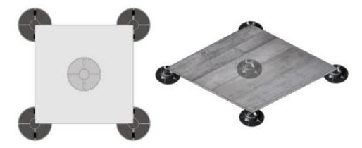
If a greater overlay height is required, Florim recommends glueing a backing plate or safety mesh to the back and additional supports under the slab, as in the attached diagram;
