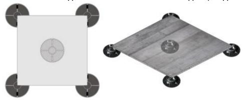
SIZE 40X120 cm: 1 support for each corner, 2 supports 1/3 along the slab and 2 supports half-way along each of the two long sides (4 supports per piece)
