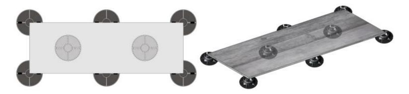
If a greater overlay height is required, Florim recommends glueing a backing plate or safety mesh to the back and additional supports under the slab, as in the attached diagram;
