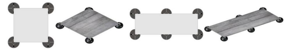
In the case of flooring for public use or where there are high loads, Florim recommends the adoption of additional supports under the slab, as in the diagram below
